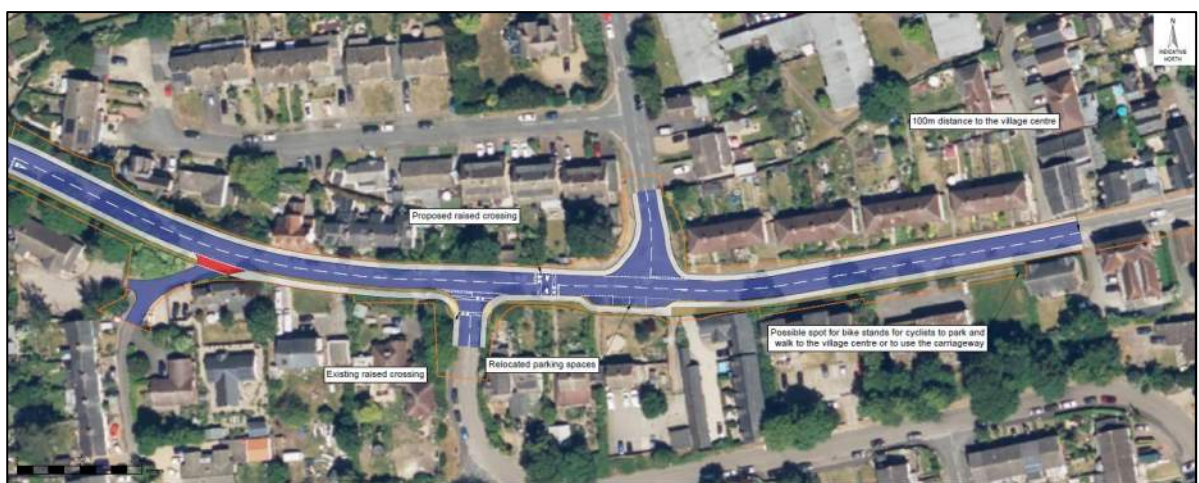
Figure 5.8 – Proposed Off-Site Improvements – B1038 Baldock Road (East)
